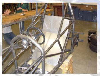
then mounted shortly after. Our battery mount, master cylinder, and nose cone housing is unique compared to the other cars but we hope that it will be a lot more efficient. The pedals were designed on Inventor and cut on the water jet at NWTC. The differential came through the mail and we were able to figure out where it needs to go along with the engine. The back end then was assembled and
